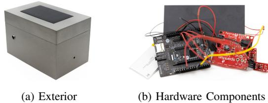
Fig. 3: Prototype of the raven deterrent system.
