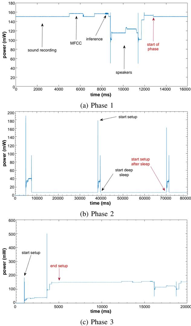
Fig. 5: Power profiles of the prototype system for each phase.
